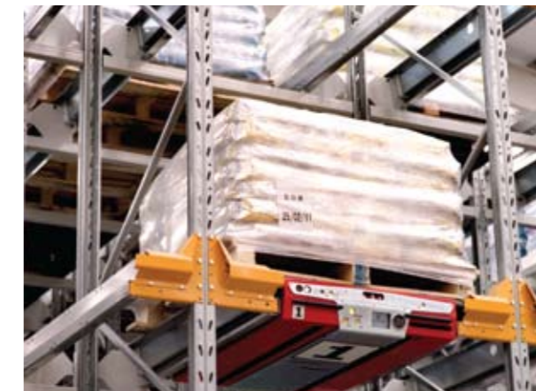
BT Radioshuttle units emit visual and audio signals when moving
