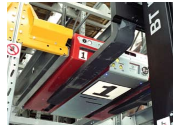
Fork guides ensure safe, accurate transfer of shuttle units using conventional forklifts
